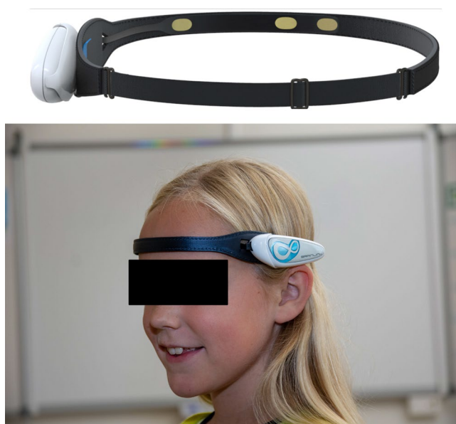
FIGURE 1 The wearable electroencephalographic (EEG) device used in this study. The dry EEG electrodes in the elastic headband are placed close to the standard EEG locations F7 and Fp1 (bipolar channel). The third electrode is the ground (at Fpz location). The device is connected to a smartphone via Bluetooth
